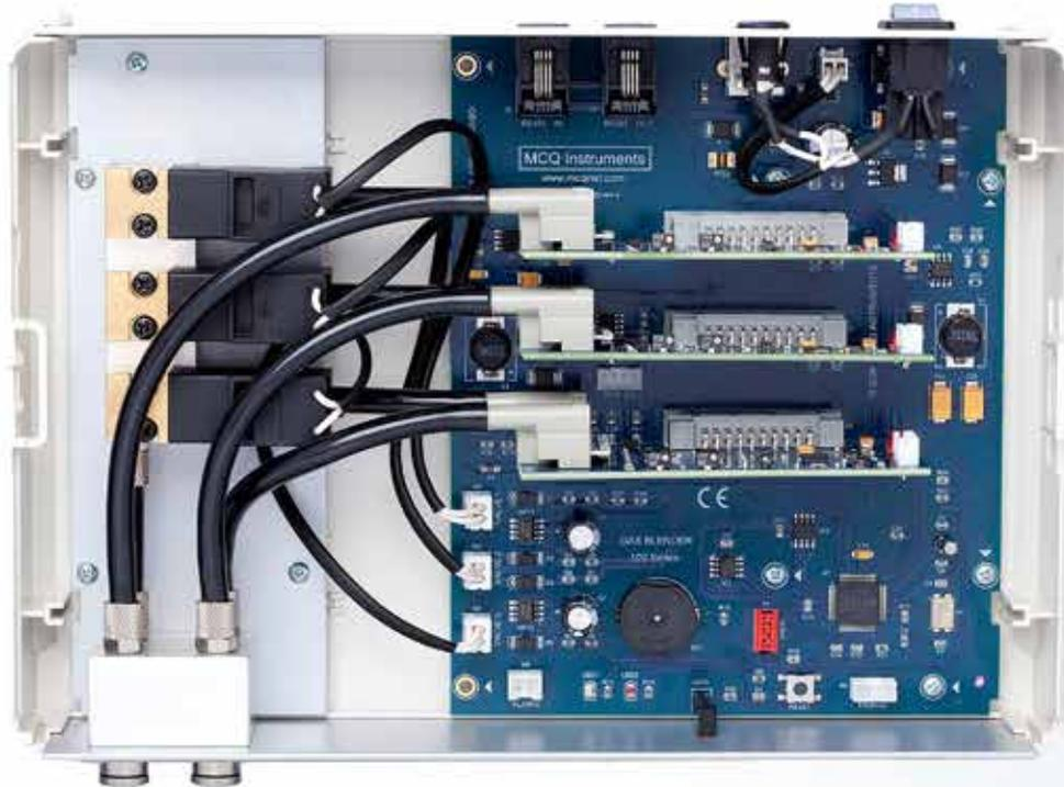
The MCQ Gas Blender 100 Series is the solution for non-aggressive gas mixing and gas dilution problems. Instead of multi-channel solutions using mass flow controller and external power supply and readout, MCQ Instruments offers a three-channels gas mixer solution in a compact box at a very convenient price (**Lab in a Box**).
