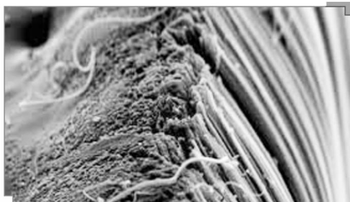
High magnification carbon nanotubes micrograph
